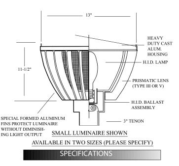
LuminaireName:LaBreaDescription:Vandalstyleluminaireconsistingofaluminumvandal<br/>proof fins and integral ballast assembly with prismatic lens.
