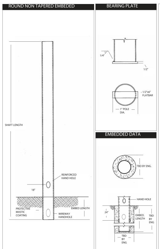
Steel poles are designed for the combined effects of both wind and dead load. The wind load effects have been analyzed with wind velocities ranging from 70 to 120 mph plus a 1.3 gust factor. Due to varying wind effects, height correction factors and drag coefficients have been applied to the entire structure. The dead load effects have been determined by using a final deflected position analysis to account for secondary moments eauentriaydead loads.
